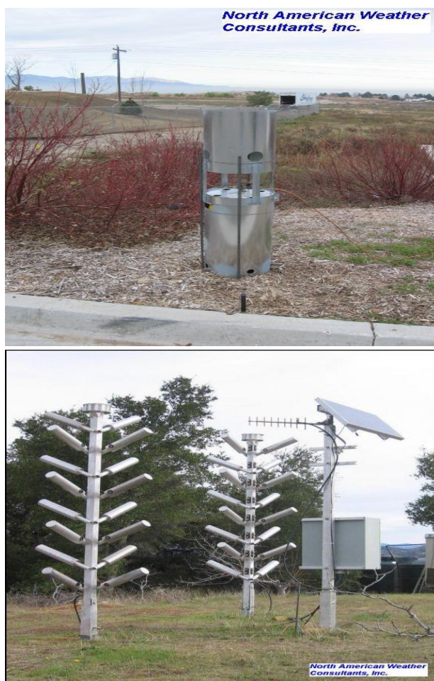
Figure 1: Photos of ground-based cloud nucleating generators. Courtesy North American Consultants Inc.
