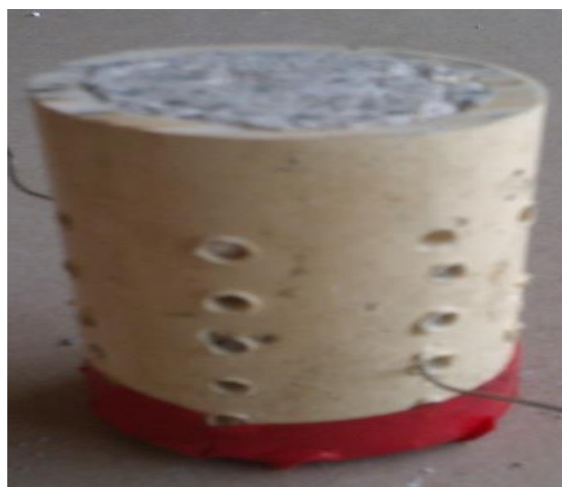
Figure 4: Perforated pyrotechnic cartridge case made up of PVC.
