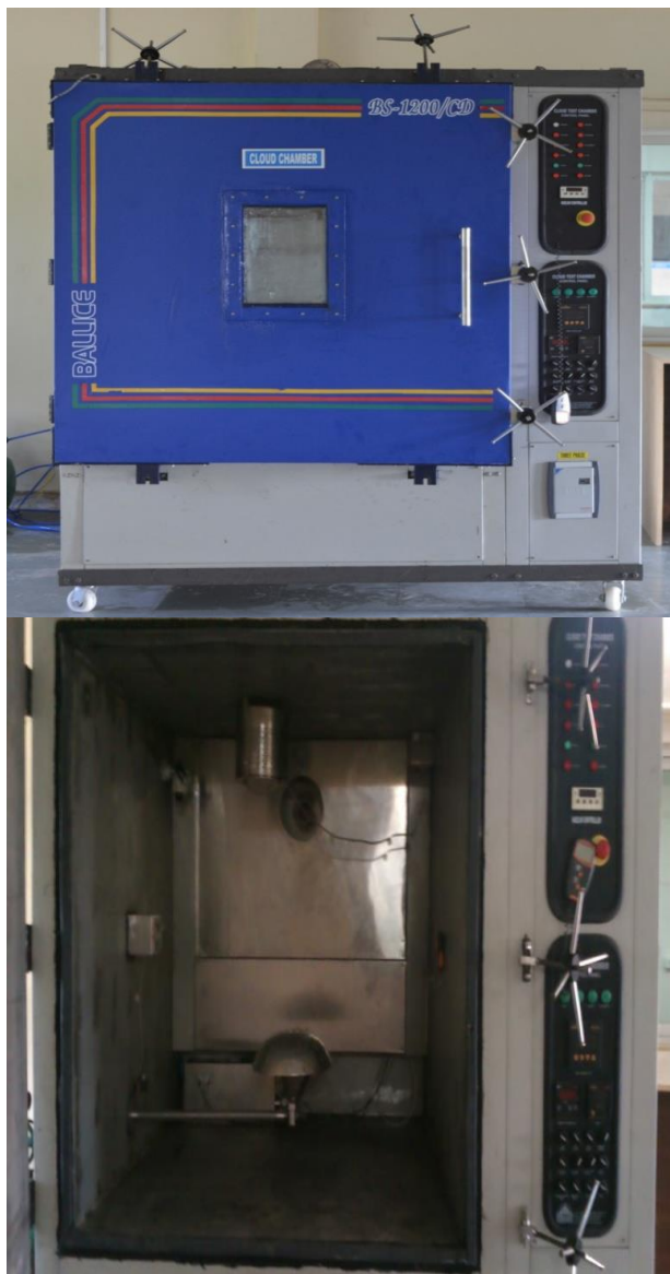
Figure 8: Cloud chamber designed and developed under NICRA project. Top is closed chamber and bottom is open chamber.
