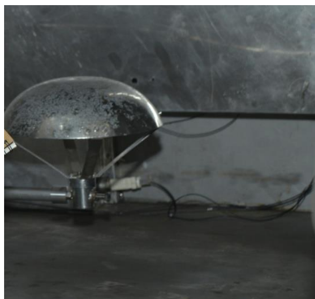
Figure 9: Silver iodide cartridges testing (fume generating) device present inside the cloud chamber.
