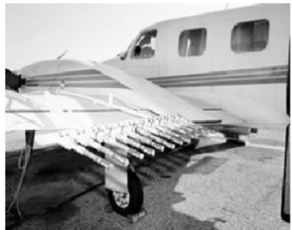
NaCl Flame generator mounted below the wings of the aircraft
