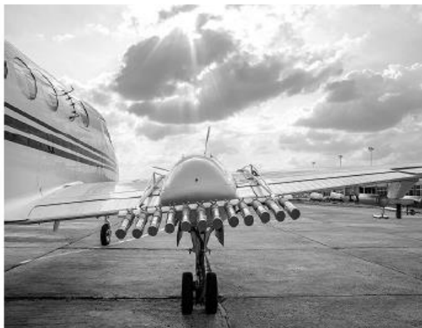
AgI Flame generator mounted below the wings of the aircraft
