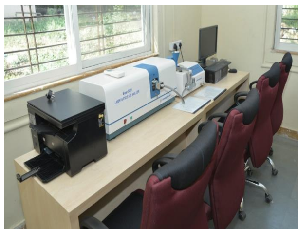
Figure 5: Particle Size Analyzer (PSA) Sizer 3002. Measuring range: 0.02 \mu m to 2000 \mu m Accuracy: \leq 0.5%. Typical measurement time: \leq 10 second.
