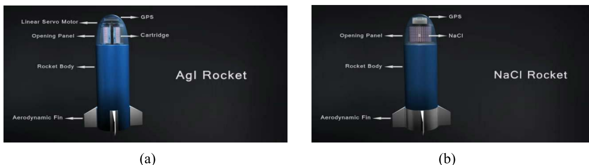
Figure 9: (a) AgI and (b) NaCl Rockets
