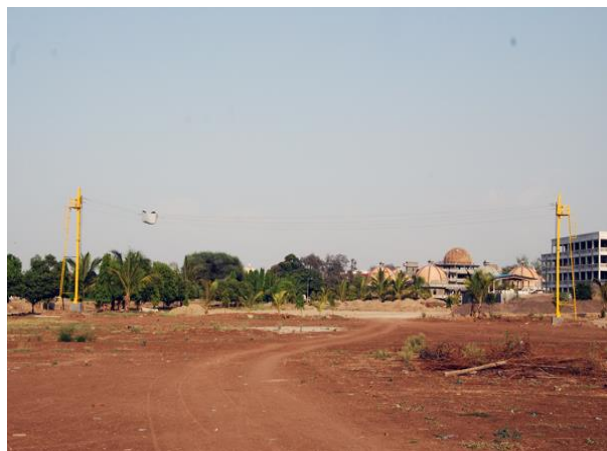
Figure 6: A live picture of the Artificial Cloud Target for Radar (ACTR) on wire supported by two yellow pillars on either side.
