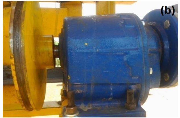
Figure 9: Two-HP forward/reverse geared motor.
