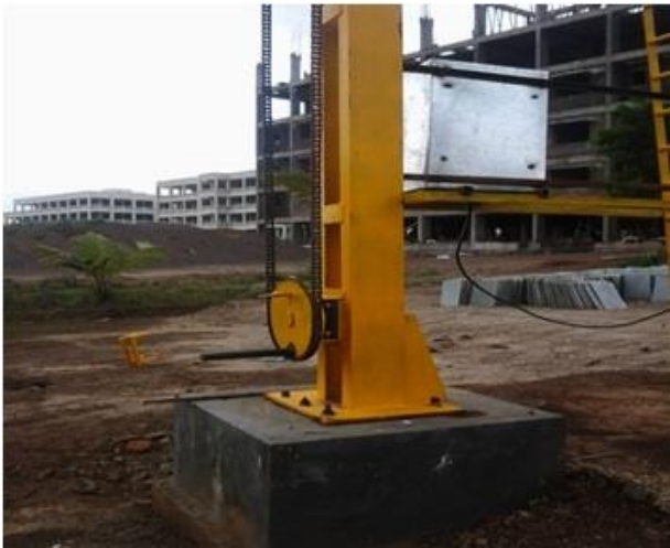
Figure 8: Toothed wheel with handle for manual rotation.
